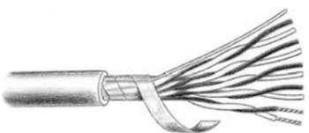
Multipairs of stranded 16/0.2mm dia conductors FR PVC insulated. Pairs numbered and twisted. Pairs laid up and overall screened with Mylar\* aluminium tape in contact throughout by a bare tinned copper drainwire and FR PVC sheathed.
