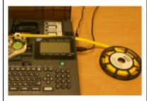
Alternative 2: Feed the profile trough the printer so that it prints on the side that **doesn't** face the reel core. (See the example below)
