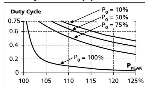
$$\text{DutyCycle} = \frac{T_{\text{peak}}}{T_{\text{peak}} + T_0}$$
