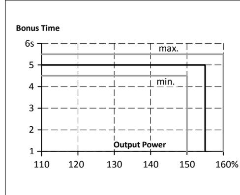
Fig. 6-3 **Dynamic overcurrent capability, typ.**
