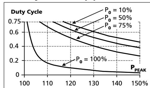
$$\text{DutyCycle} = \frac{T_{peak}}{T_{peak} + T_0}$$
