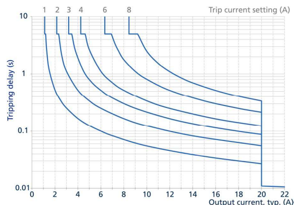
Fig. 6-2: Tripping delay depending on current slow tripping characteristic
