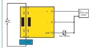
**Note!,** Using the digital output only – the negative DC supply must be connected to terminal 8
