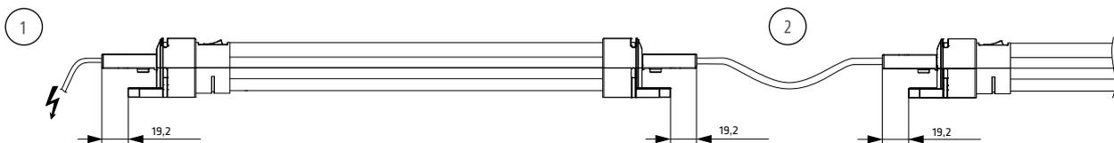
This illustration shows the LED 021/022 lamp in a daisy chain application. The lamps are conveniently connected via connection plugs - up to 8 lamps max. can be daisy-chained this way. The snap lock connectors ensure a stable electrical connection even if subjected to heavy vibration. The connection example shows a AC 230 V application, using the following cables: connection cable with female connector, Art. No. 244356 (1); daisy chain extension cable with 2 connectors, Art. No. 244358 (2).
