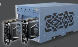
Nuvo-8208GC is the first of its kind to offer such stellar CPU/ dual GPU tandem and computational power in an industrial-grade rugged compact design. Its rich I/O ports can be easily accessed and accepts a wide-range DC input (8~35V) making it easy to deploy and extremely flexible for all your critical industrial Al applications.
