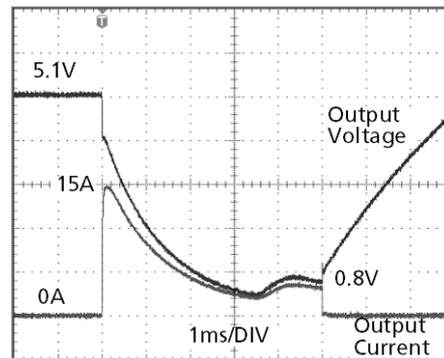
Peak load 15A (resistive load) for 5ms
