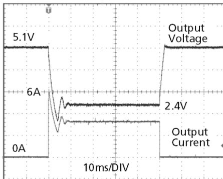
Peak load 6A (resistive load) for 50ms
