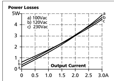
Fig. 8-3 Efficiency vs. input voltage at 5V, 3A, typ.
