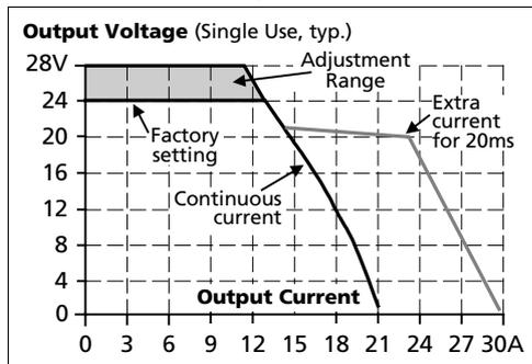
Fig. 6-2 **Output voltage in "parallel use" mode, typ.**
