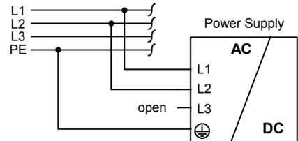
Fig. 22-6 **Allowed output current for use on only two legs of a 3-phase system**
