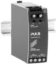
The YR80.242 is the preferred redundancy module for the CPS20.121 power supply. It is equipped with two input channels, which are individually decoupled by utilizing mosfet technology. Using mosfets instead of diodes reduces the heat generation and the voltage drop between input and output. The YR80.242 does not require an additional auxiliary voltage and is self-powered even in case of a short circuit across the output.
