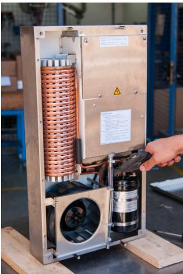
e. Spray cleaning fluid onto a cloth and wipe down unit
