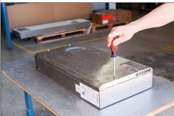
b. Remove the cover of the controller box
