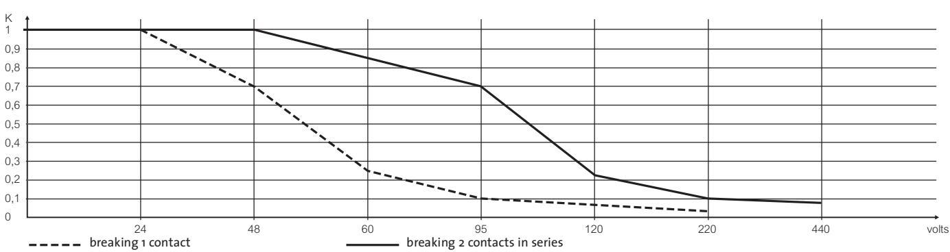
reduction coefficient K for rated operating current in DC-1 continuous current
